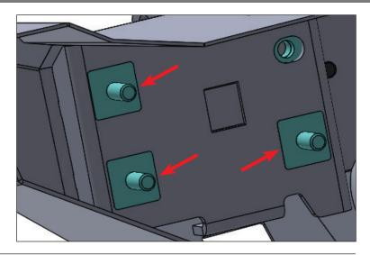
5. Now lift and place the bumper to the Jeep frame rails. The studs slide through the holes in the frame holes. It's best to have an assistant to lift and hold the bumper in place.
