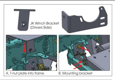
11. Now install passenger side JK winch bracket. Slide T-nut plate into the frame slot (see image A). The bracket mounts to the winch tray with two M8 bolts with flat, lock washers and nuts. Next mount to the Jeep frame with M10 bolt and flat washer to the T-nut plate in the JK frame (see image B).
