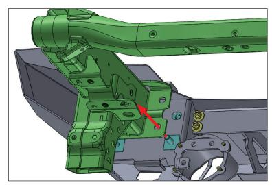
6. With bumper in place thread the hardware to the bumper. On the inside upper location it takes M12 bolt with flat and lock washer. The other three mounts use M12 nut with flat and lock washer. Do not tighten at this time just hand tighten to hold bumper in place.
