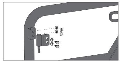
3. Using caution, slowly insert Tube Door in door hinges and reinstall factory door nuts.
