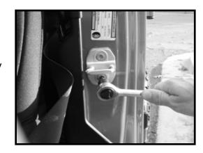
8. Attach Nylon Door Strap to the door hook located at the lower front corner of the inner Half Door. Loop the other end around the factory hook inside the vehicle floor compartment. Replace plastic cover.
