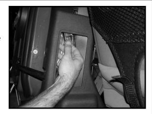
2. Remove the torx nut from the bottom of each factory hinge pin. Set these nuts aside to be re-installed on the Half Doors. To remove the factory doors, carefully lift the door upward until the hinge pins completely clear the hinges. It will be helpful to have someone else assist with this step.
