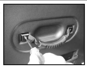
5. Install doors by aligning the door hinge to the holes of the vehicle hinges. Do not force the alignment. It may be necessary to carefully swing the door back and forth several times to allow the hinges to properly seat. Install torx nuts removed in step 3. Tighten to 7 ft-lbs. **NOTICE!** Do not attempt to close door before making adjustments detailed in the next step.
