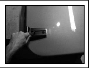
4. Attach the Grab Handle to the door using Grab Handle Mount Plates and M6 Bolts by carefully aligning with threaded hole locations on door.
