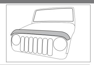
1. Clean and open hood. Test fit bug deflector centrally on hood. Note (2) holes in hood cooresponding with two slots in bug deflector. Remove bug deflector. Insert plastic screw plugs into holes previously noted.
