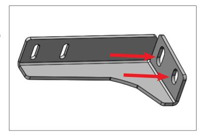
2. Now feed the upper bracket between the bumper and body. Once you have the upper and lower bracket meeting attach the two items with the provided carriage bolts and serrated flange nuts. Fully tighten all hardware.
