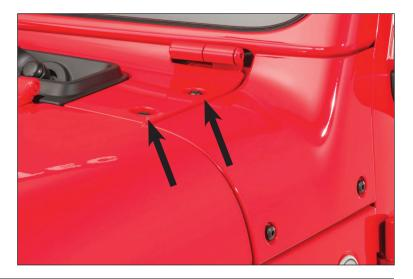
2. To install the LED mount bracket place the thicker 2.8mm stainless washer in front cowl location and the thinner 1.5mm stainless washer in the rear cowl position. Now place the plastic spacers on top of the stainless washers. Place bracket on top of the spacers and feed the Button head bolt and washer (provided) through the bracket and spacer to the threaded hole. Tighten to secure, **DO NOT over tighten or use power tools to tighten**.
