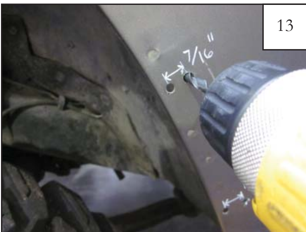
Using a 1/4" drill bit, drill marked holes.
