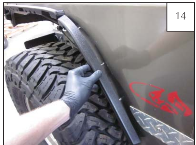
Secure inner piece D2 (and P2 for passenger side installation) to the sheet metal using the following 2 Steps: Step 1 Line up the three Screws (SW1-0053) with the upper factory hole and two drilled locations.
