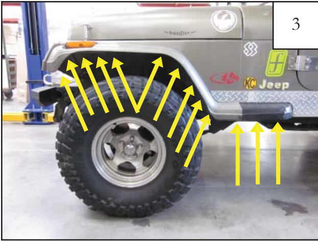
Remove the factory installed fender flare and rocker guard screws with a socket wrench. (12 total locations) 9 on main flare (use 5/16" socket), 3 on rocker panel (use 3/8" socket)
