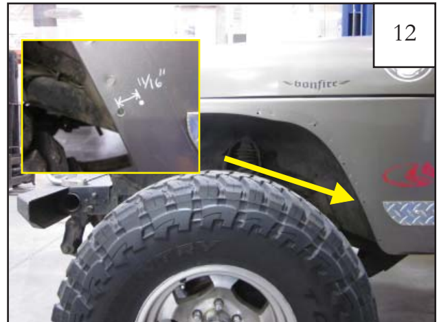
Locate the second factory hole from bottom of fender. Use a grease pencil to mark a hole for drilling 11/16" from center of factory hole, perpendicular with wheel well opening.
