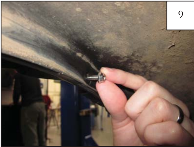
Step 2 Attach Nuts (NU1-0010) to the threads on the Screws (SW1-0053) and hand tighten.
