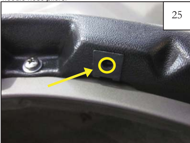
Before installing the outer flare, make sure that the Clips (CL1-0022) on the inner pieces are centered over the predrilled holes.
