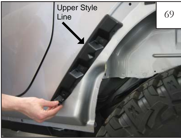
Step 2 While holding the inner piece in place, install a plastic push retainer in each hole location. Inner piece should rest along upper style line of sheet metal radius and not below it: see step 22. NOTE: Foam insulation may need to be trimmed out of the holes.
