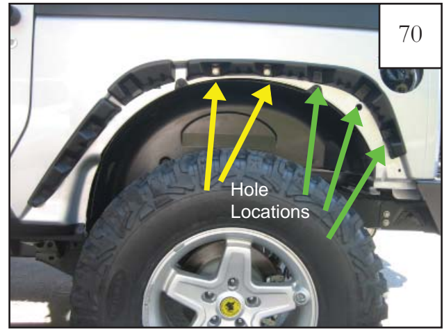
Secure inner piece D4 (and P4 for passenger side installation) to the sheet metal using the following 4 STEPS: Step 1 Position inner piece on fender, aligning with existing factory holes in sheet metal.
