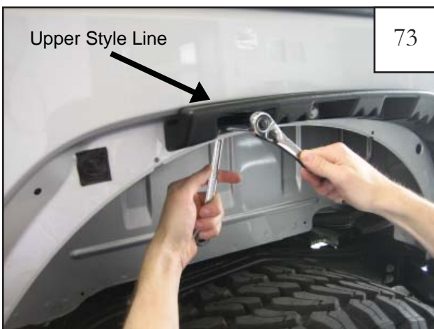
Step 4 Using a 1/2" socket wrench and a 1/2" wrench, tighten all bolts until inner piece is snug against fender. Do not overtighten: see step 21. Inner piece should rest along upper style line of sheet metal radius and not below it: see step 22.
