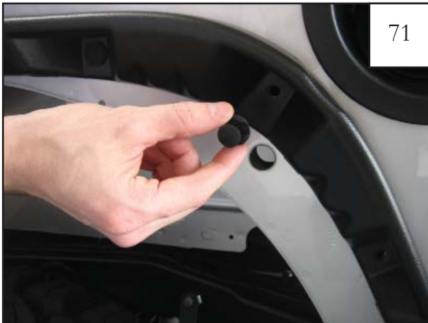
Step 2 While holding the inner piece in place, install a plastic push retainer in the rearward three hole locations.
