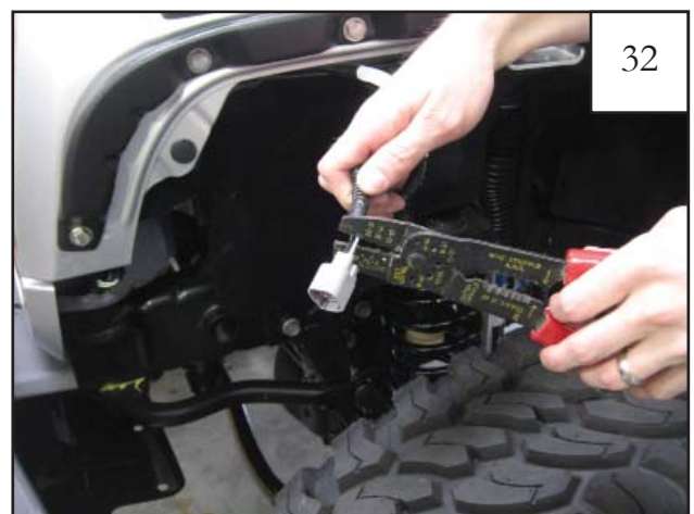
Use wire cutters to cut the two wires at the base of the factory side marker lamp.
