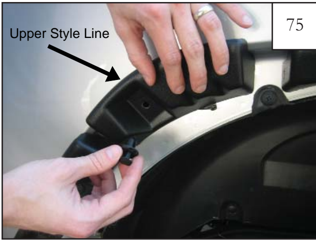
Step 2 While holding the inner piece in place, install a plastic push retainer. Inner piece should rest along upper style line of sheet metal radius and not below it: see step 22.
