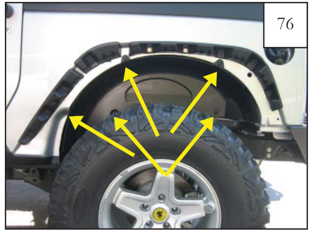
Reinstall modified splash shield using supplied 1/4" Plastic Retainers (5 locations).
