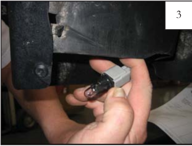
Remove light receptacle from light lens housing, letting it hang free of the housing.
