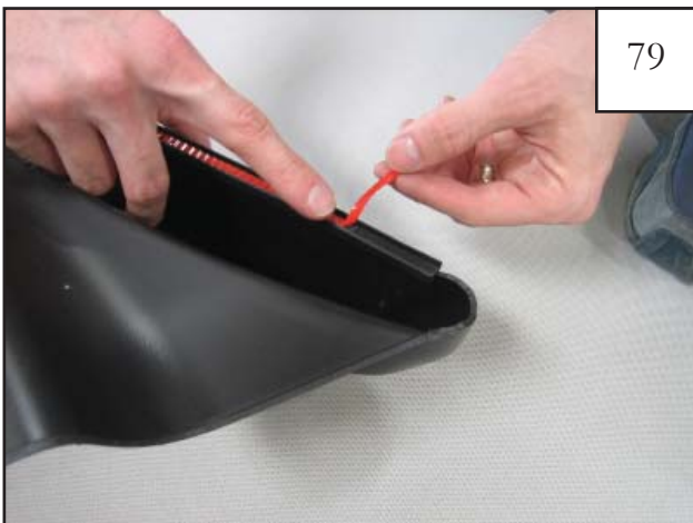
Peel back 1-2" of red liner on each end of the edge trim and bend toward the outside of the flare.
