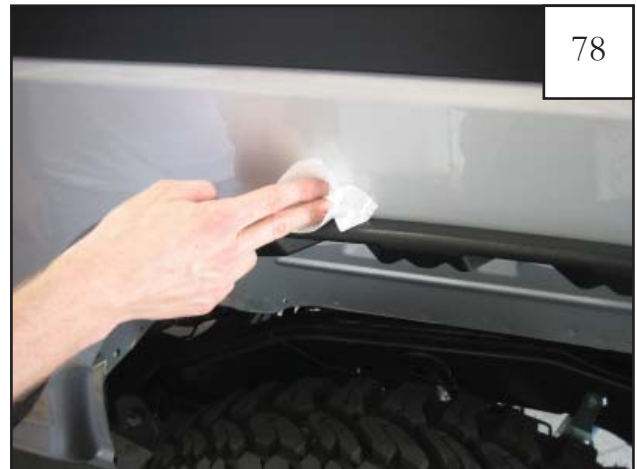
Use one supplied alcohol prep pad to clean the sheet metal above each inner piece in preparation to tape the edge trim to the sheet metal. This must be done for proper flare installation.
