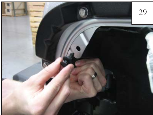
Reinstall inner splash shield by first placing a supplied plastic push retainer through the mounting hole in the sheet metal and splash shield as shown in picture. Note: Splash shield should be behind sheet metal.
