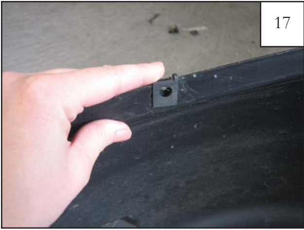
Install supplied #14 U-Clips over existing holes in splash shield (6 places). Flat side will be visible once splash shield is reinstalled.
