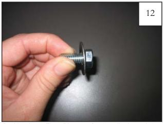
Position Inner Flare Piece on fender, aligning existing 5/16" holes in Inner Flare Piece with holes on fender. Slide a supplied 1" Fender Washer onto supplied Hex Head Bolt.
