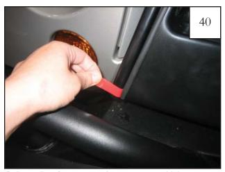
Pull tape liner from tape and press part to vehicle to secure adhesive backing. Tighten all Truss Head Screws first, then tighten all Torx Screws, moving from back to front.
