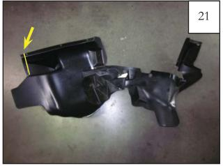
Using a grease pencil make a mark in 1" from edge of factory sheild and up to top edge of part where holes are located.
