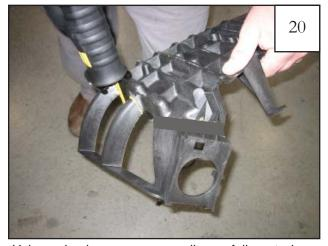
Using a hacksaw or a sawsall, carefully cut along lines made in Steps 19 and 20 to remove from portion of factory inner structure. Keep the rearward peice and set aside.
