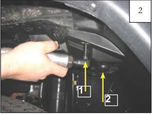
Using a socket wrench with a 10mm socket, remove bolt located in hole inside of splash shield (location 1) and bolt in location 2. Save fasteners for reinstallation. Note: 2007-2010 model years have a plastic thread engager in location 2. Remove and save for reinstallation.
