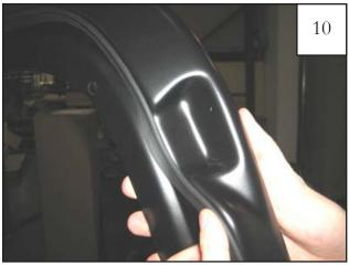
When positioning gimp around latch section for front, make sure round edge of gimp is positioned below the egde of the part (Gimp will continue over entire length of part).
