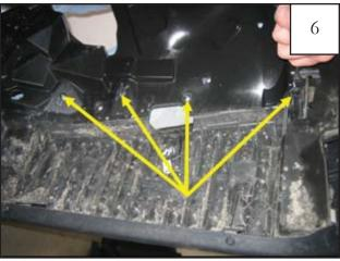
To remove inner structure and splash sheild from factory flare, use pry tool or flat head screwdriver to remove four plastic fasteners.
