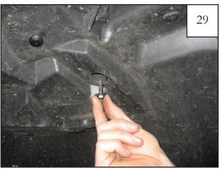
Reinstall the factory bolt through hole in splash sheild as shown.
