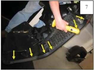
Use a drill with a 5/16" bit to drill through six plastic riviets along edge of flare/splash sheild. Discard the flare, but retian the splash shield and inner structure.
