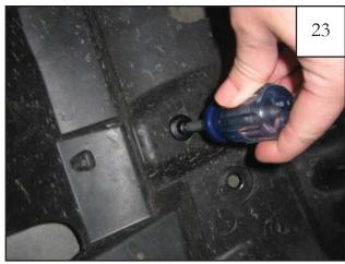
Using a Phillips screwdriver, reassemble inner structure and splash sheild by installing supplied Plastic Phillips Head Tufloks (6 places). Use a pushing-twisting motion to install.
