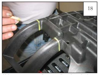
Using a grease pencil, trace a line along the base of the first and second spines of the factory inner structure as shown. This line will be cut in Step 20.
