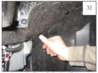
Install a supplied Plastic Phillips Head Tuf-lok in hole located towards the front of the splash sheild.
