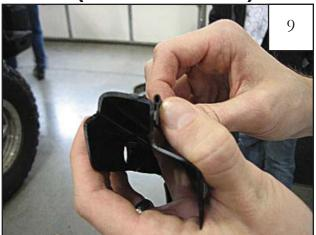
Make sure gimp and inner flare are clean. Peel 2" of liner from gimp (pin shape). Carefully position gimp as uniformly as possible along radius as shown, peeling liner as you go. Gimp can be repositioned as needed. Note: It is better for gimp to be slightly below the radius rather then above.
