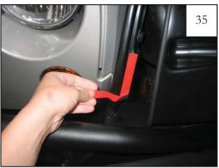
Fold tape liner tab attached to 1/2" peice of tape on outer edge of Inner Flare Piece upwards (do NOT peel liner from 1/2" tape in this step).
