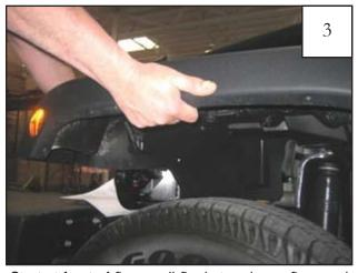
Start at front of flare, pull firmly to release flare and splash shield from fender, working your way to the back. You will hear popping noises as clips release. it is okay if the clips break, they will be discarded.
