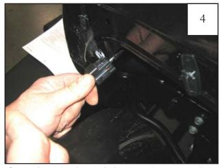
Once flare is free of fender, disconnect light connector. this will allow the flare to come away from fender completely. Remove light housing from factory flare; you will be reinstallaing this later.
