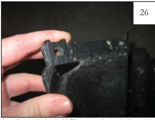
Install supplied #14 U-Clips over holes indicated in Step 27.
