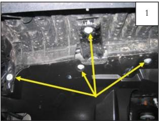
Using a socket wrench with a 10mm socket, remove four factory bolts from inside of splash sheild. Set bolts aside for reinstallation.
