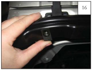
Install supplied "U" Nut, with the thread side in, over holes in Inner Flare Piece (8 places). Make sure nuts are centered over holes.
