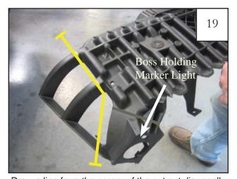
Draw a line from the corner of the cut out diagonally across the ribs of the factory inner structure as shown. Note: Line placement can vary 1/2" inch in either direction from shown. **DO NOT CUT OFF BOSS HOLDING MARKER LIGHT.**
