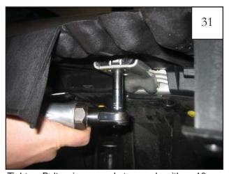
Tighten Bolt using a socket wrench with a 10mm socket.
